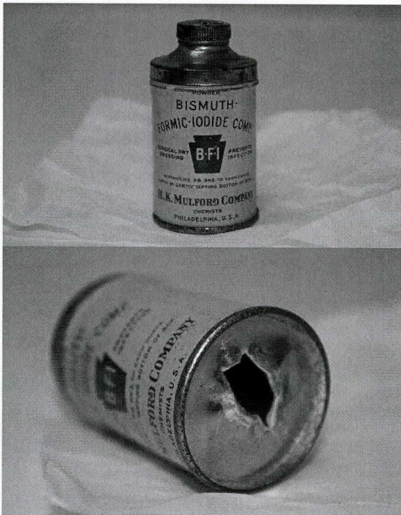
Figure 3. Hole cut in the bottom of a metal container in order to remove the contents while maintaining display value.
