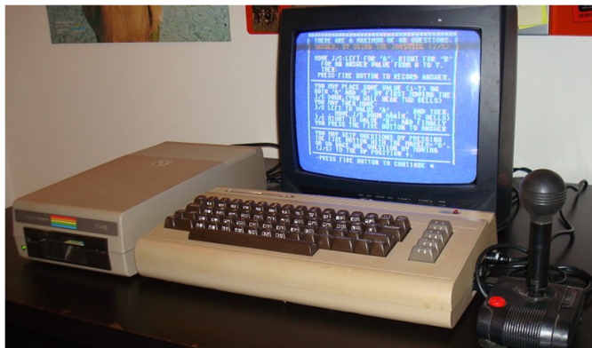
Fig. 1. Commodore 64 hardware C64 setup (from left to right): VIC-1541 Drive, C64 computer, vision monitor and joystick
